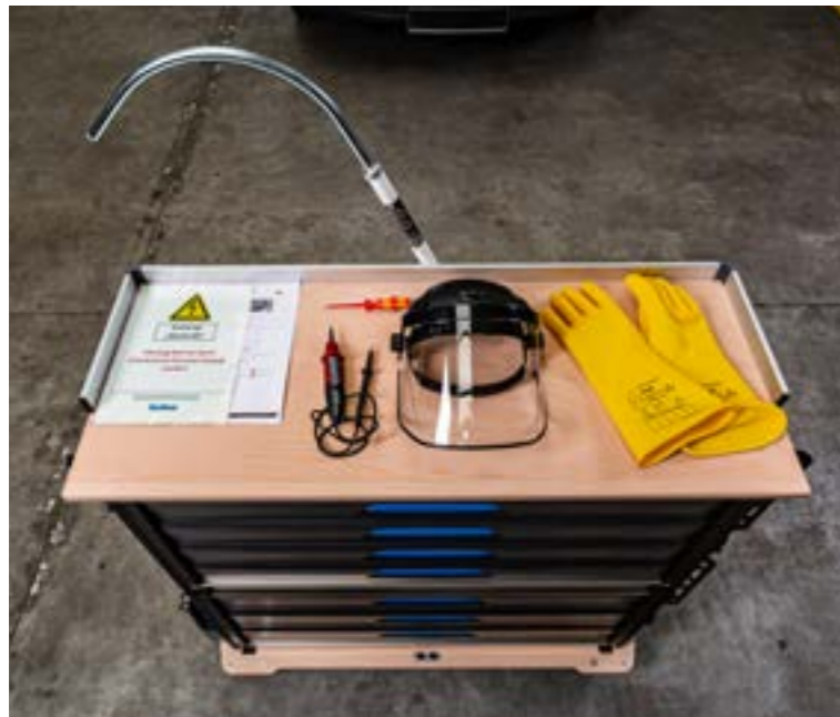
Mobile high-voltage workplace
